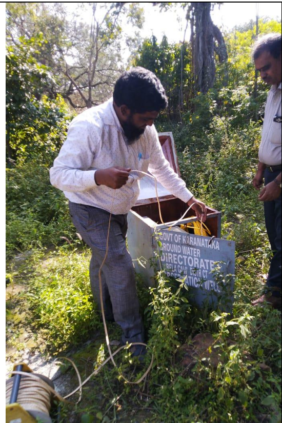
8. Measuring Groundwater Head at Bailhongal Observation bore well
