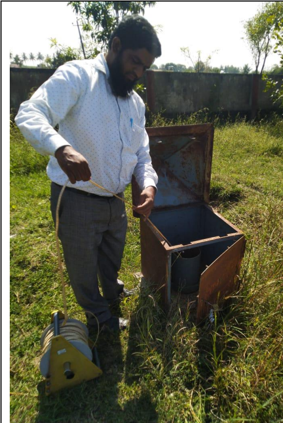
5. Measuring Groundwater Head at Chikkabagewadi Observation well
